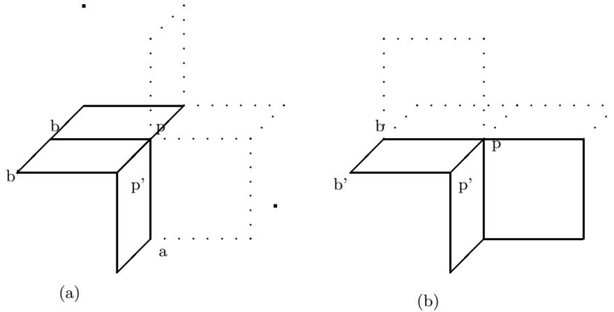
Fig. 5.13. Two cases that can be developed.
